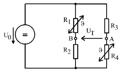
Werte:  $U_0 = 30V$ ,  $R_1 = 10k\Omega$ ,  $R_2 = 20k\Omega$ ,  $R_3 = 50k\Omega$ ,  $R_4 = 100k\Omega$ ,  $\alpha = 0.01K^{-1}$
