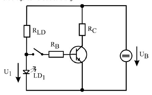
Werte:  $U_B = 25V$ ,  $R_C = 500\Omega$ ,  $R_B = 28k\Omega$ ,  $R_{LD} = 1k\Omega$ ,  $R_{LD} = 100$
