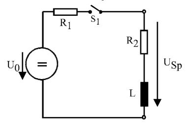
Werte:  $U_0 = 12V$ ,  $R_1 = 1\Omega$ ,  $R_2 = 2\Omega$ , L = 20mH
