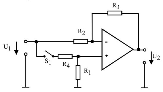
Werte:  $R_1 = 40k\Omega$ ,  $R_2 = 10k\Omega$ ,  $R_3 = 20k\Omega$ ,  $R_4 = 50k\Omega$ ,  $U_1 = 2V$
