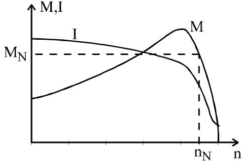
Werte:  $n_N = 1350 \text{ min}^{-1}$ ,  $U_N = 400 \text{V}$ ,  $M_N = 50 \text{Nm}$ , f = 50 Hz
