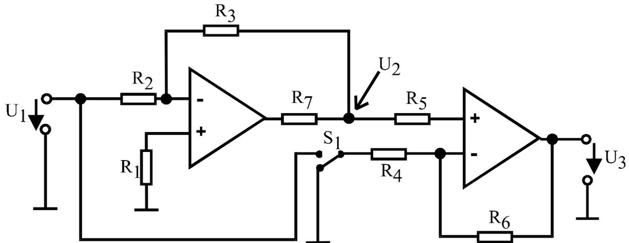
Werte:  $R_1 = 10\text{k}\Omega$ ,  $R_2 = 20\text{k}\Omega$ ,  $R_3 = 30\text{k}\Omega$ ,  $R_4 = 40\text{k}\Omega$ ,  $R_5 = 50\text{k}\Omega$ ,  $R_6 = 60\text{k}\Omega$ ,  $R_7 = 70\text{k}\Omega$ ,  $U_1 = 4\text{V}$
