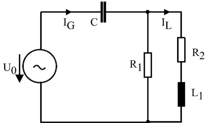
Werte:  $I_L = 1\text{A}$ ,  $R_1 = 100\Omega$ ,  $R_2 = 100\Omega$ ,  $L_1 = 160\text{mH}$ ,  $C = 64\mu\text{F}$ ,  $f = 50\text{Hz}$
