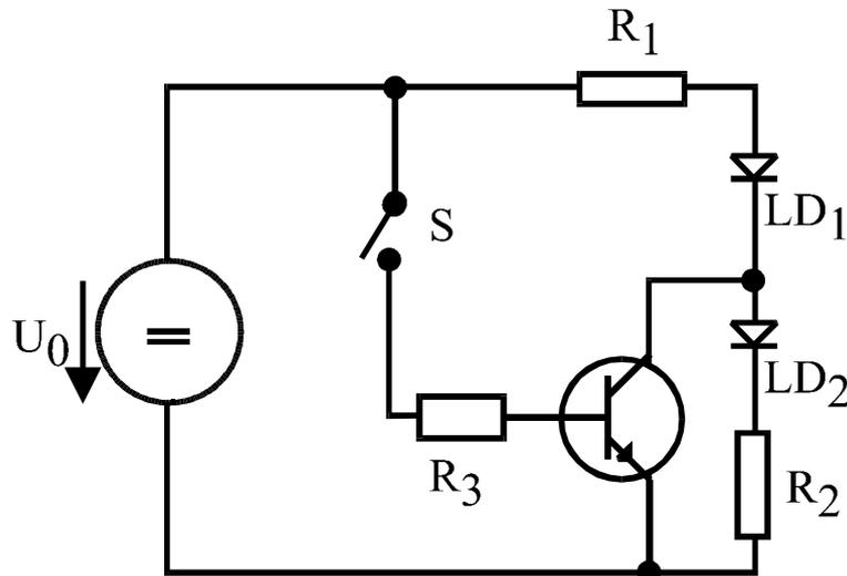
Werte:  $R_1 = 300\Omega$ ,  $R_2 = 200\Omega$ ,  $U_0 = 10V$ ,  $R_3 = \text{z.B. } 1k\Omega$
