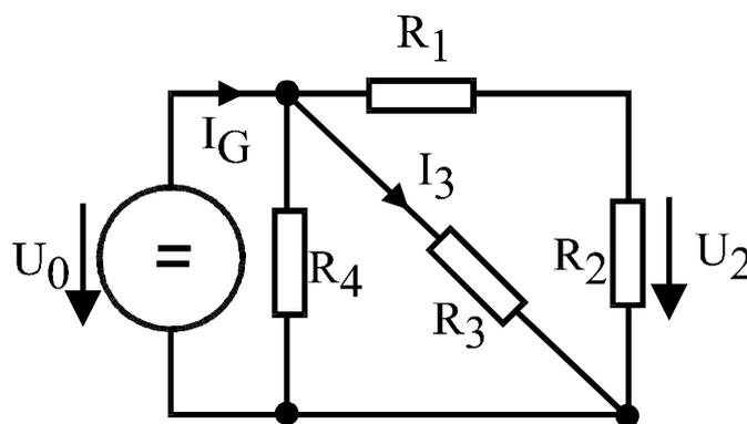
Werte:  $U_2 = 2\text{V}$ ,  $R_1 = 10\Omega$ ,  $R_2 = 20\Omega$ ,  $R_3 = 30\Omega$ ,  $R_4 = 40\Omega$ ,
